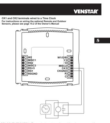
DRY CONTACT SWITCH - The terminals are 'normally open' (may be programmed for normally closed operation, see page 16.2 of the Owner's Manual). Closing or completing the circuit will cause the thermostat to do one of the following:
