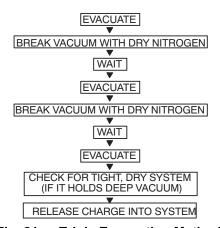
Fig. 21 — Triple Evacuation Method
