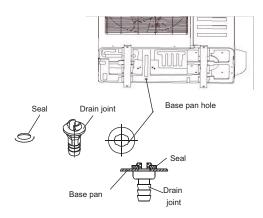
Fig. 10 — Drain Joint
