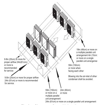
Fig. 8 — Clearances for multiple units
