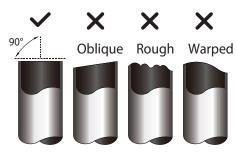
Fig. 11 —Pipe Cutting
