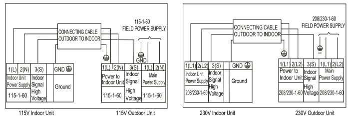
Fig. 23 —Connection Diagrams
