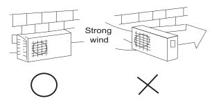
Fig. 9 — High Wind Installation
