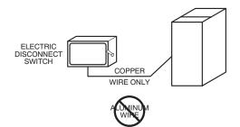
Fig. 33 – Field-Supplied External Electrical Box on Furnace Casing J-Box Installation
