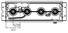
Fig. 70 – Igniter Position - Top View
