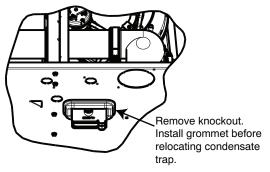
Fig. 17 – Horizontal Drain Trap Grommet
