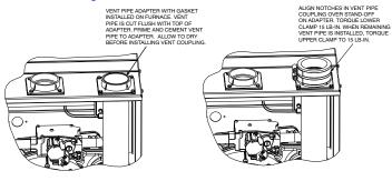
VENT PIPE FLUSH WITH ADAPTER
