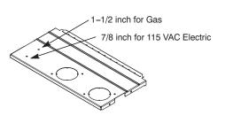
Fig. 30 – Alternate Gas and Electric Entry A170125
