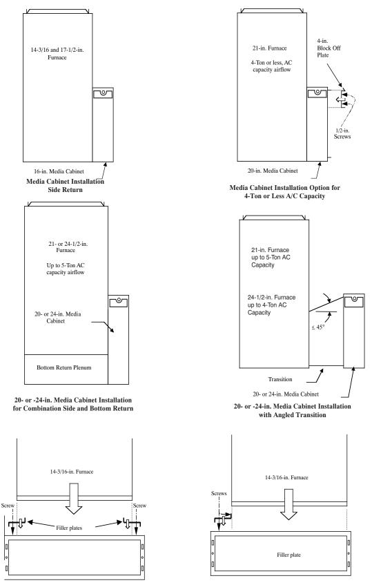
14-3/16-in. Furnace with Filler Plates, Off-Set to Right
