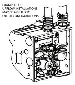
Fig. 50 – Sample Inlet Air Pipe Connection for Polypropylene<sup>A12220</sup> Venting Systems
