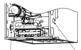
Gas Pipe Grommet Required For Direct Vent Applications Left Side Gas Entry. Gas Pipe Grommet Required For Direct Vent Applications.
