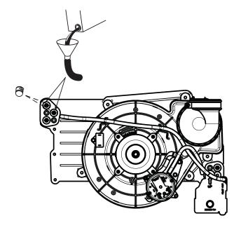
Fig. 61 – Priming Condensate Trap (Appearance May Vary)
