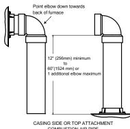
COMBUSTION AIR PIPE (NON-DIRECT VENT FOR ALL MODELS EXCEPT MODULATING UNLESS INSTALLED IN ATTIC OR CRAWL SPACE)
