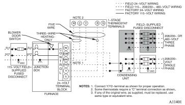
Fig. 32 – Typical Field Wiring Diagram
