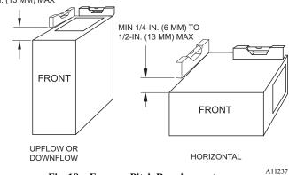
Fig. 18 – Furnace Pitch Requirements
