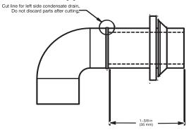
Fig. 16 - Modify Rubber Drain Elbow
