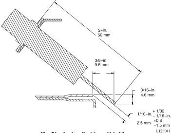
Fig. 71 - Igniter Position - Side View
