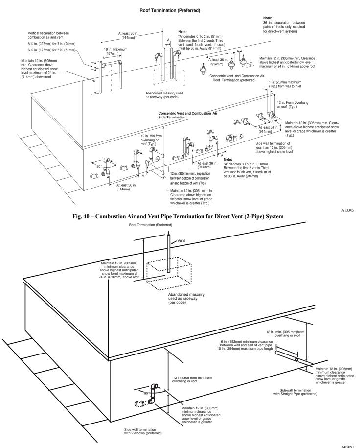
Fig. 41 – Vent Pipe Termination for Non-Direct Vent and Ventilated Combustion Air System
