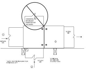
Fig. 22 – Horizontal Return Air Configurations A11038 and Restrictions
