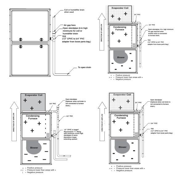
Fig. 11 – Example of Field Drain Attachment
