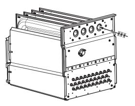
Fig. 72 – Cleaning Heat Exchanger Cell
