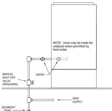
Fig. 31 – Typical Gas Pipe Arrangement
