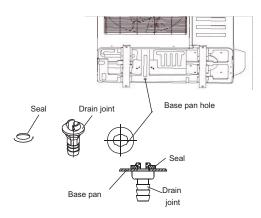
Fig. 9 — Drain Joint
