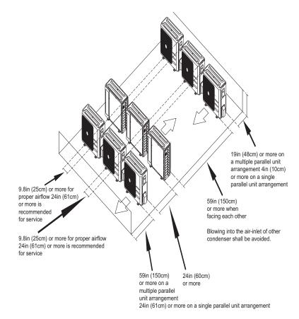
Fig. 7 —Clearances for multiple units
