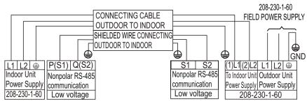
Fig. 22 — Connection Diagram Sizes 36K - 58K
