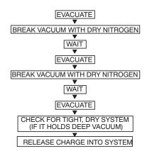
Fig. 20 — Triple Evacuation Method
