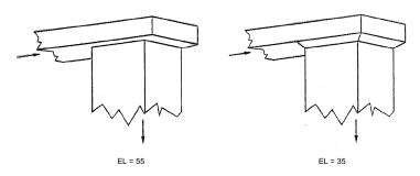
Note that the drop connection is relatively large. This was a common lowboy furnace connection.
