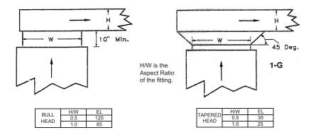
The H/W Height/Width ratio must be calculated to determing EL equivalent length.
