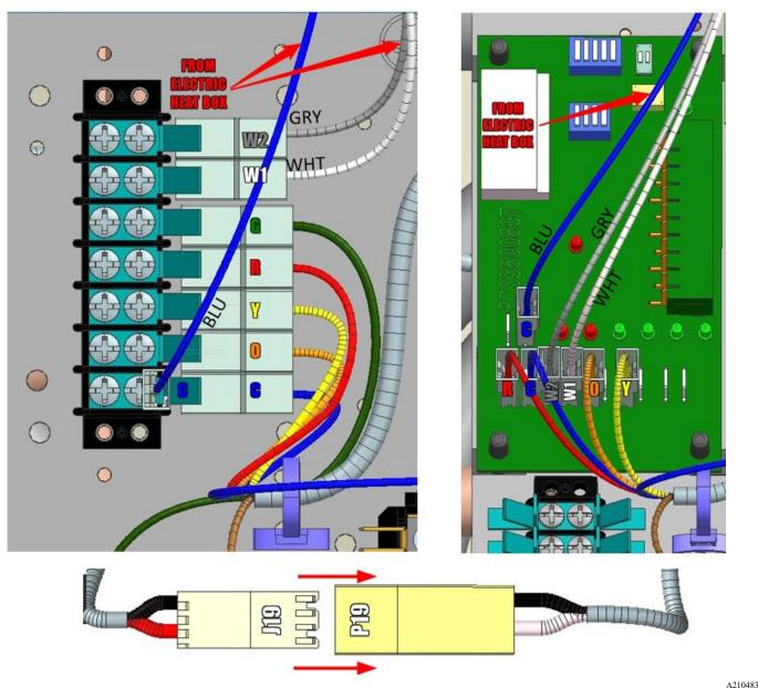
Fig. 16 – GB/HB Connections (Left), GP/HP Connections (Right), and J19 to P19 Example (Bottom). Note: Harnesses are subject to change, so your connection harness may look slightly different.
