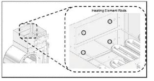
Fig. 7 – Heating Element Rods
