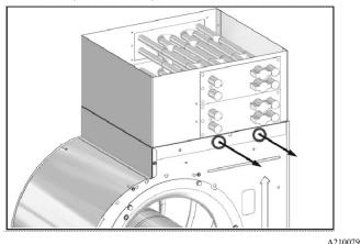
Fig. 13 - Remove Two (2) Screws
