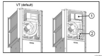
Fig. 1 – Electric Heater Element Cover (1) and Electric Heat Control Box (2) Location - Vertical Configuration
