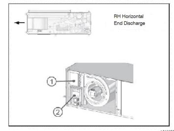
Fig. 3 – Electric Heater Element Cover (1) and Electric Heat Control Box (2) Location - RH Horiz. End Discharge Config.
