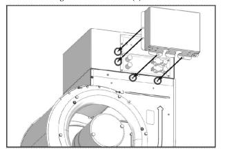
**Fig. 14 – Mount Heater Element Cover to Blower Collar** EH Control Box Installation
