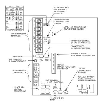
Fig. 14 - Two-stage Furnace Control
