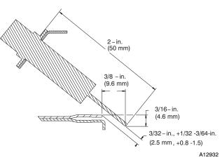
Fig. 9 - Igniter Position - Side View
