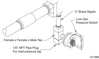
Fig. 30 - 80% Low Gas Pressure Switch
