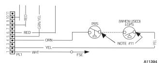
Fig. 31 - 80% Pressure Switch Wiring
