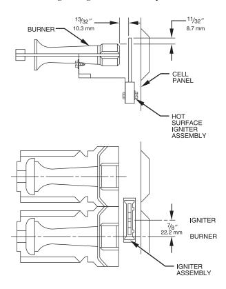
Fig. 27 - Silicon Carbide Igniters
