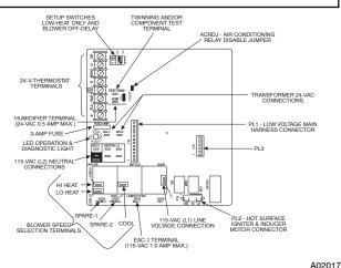
Fig. 32 - 80% Furnace Control Board
