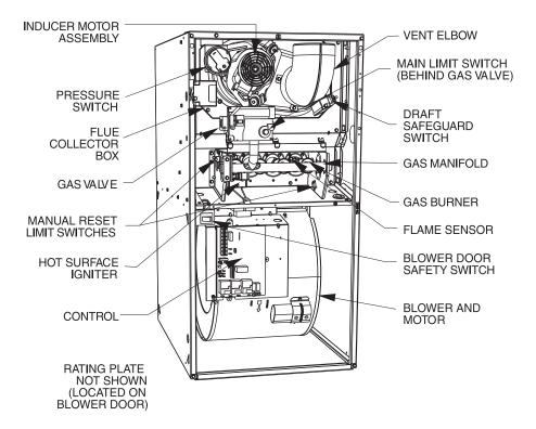
Fig. 17 - Representative Furnace Drawing
