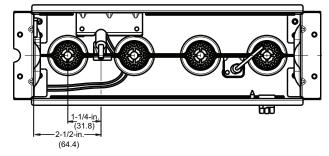
Fig. 8 - Igniter Position - Back View
