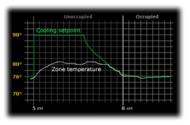
The actual equation that the controller uses to calculate **Optimal Start** is nonlinear. An approximation of the result is shown below.
