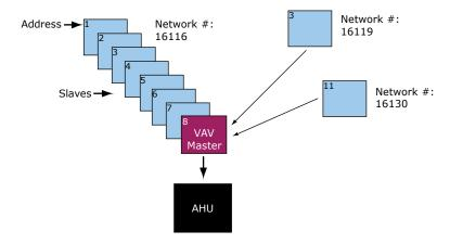
**EXAMPLE #3**: The above network plus sub-masters and their slaves. (For VAV systems only. VVT systems do not support sub-masters.) The sub-masters exchange data between their slaves and the VAV Master, and the VAV Master handles data exchange for the whole system.
