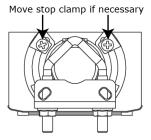
Hold down the actuator damper release button, rotate the damper to verify that it fully opens and closes, then release the button.
