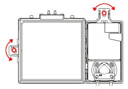
4 Hold down the VAV Zone II's actuator release button and rotate the actuator clamp in the same direction that closed the damper. Rotate the clamp until it stops, then rotate it back one notch.
